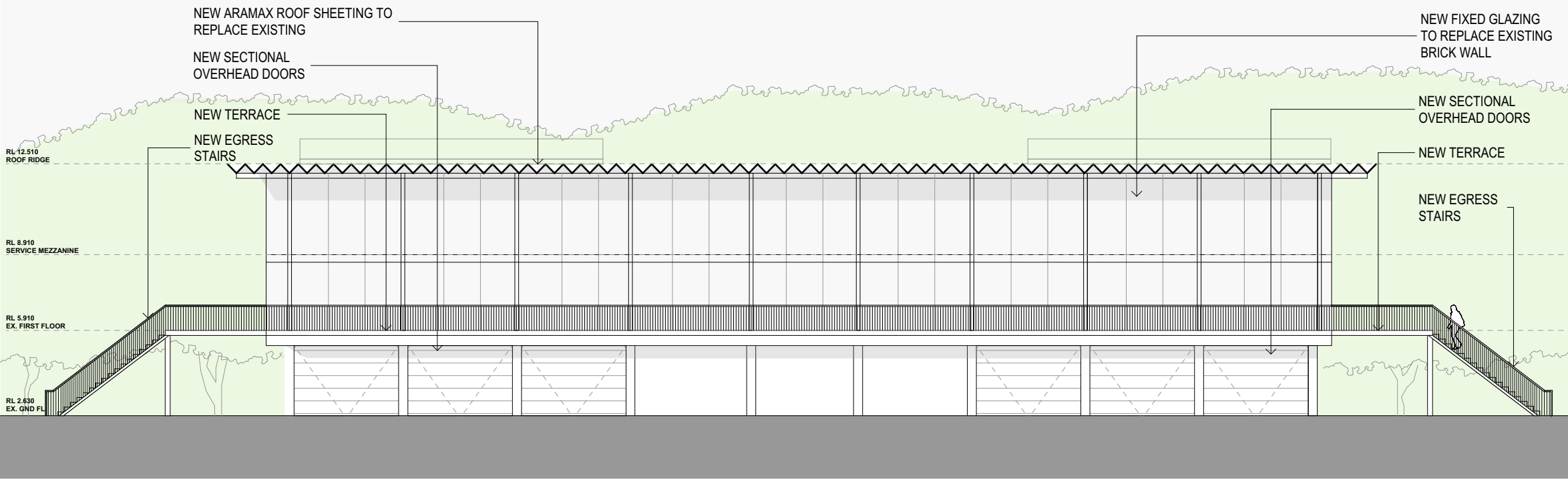
Proposed West Elevation 1:200
